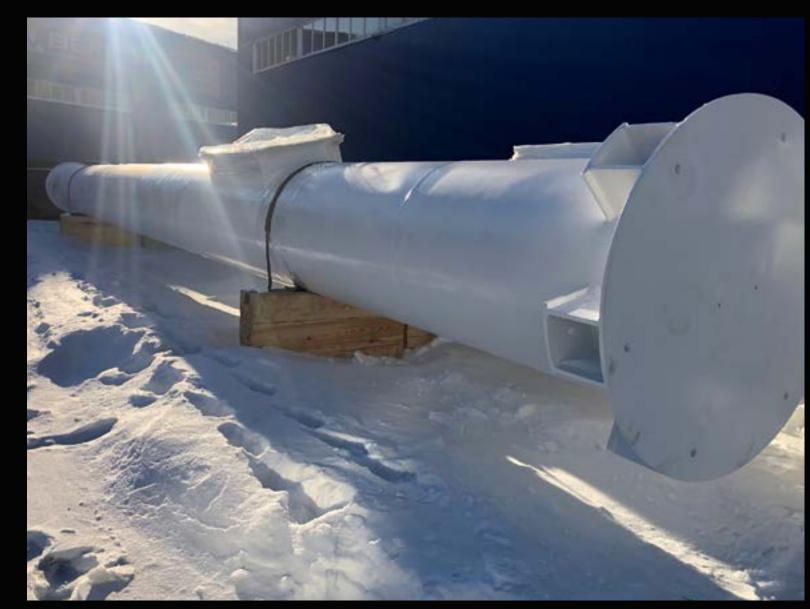
Production of air-intake pipes for ensuring fresh air supply to the facilities of Irkutsk Polymer Plant (the town of Ust-Kut).
