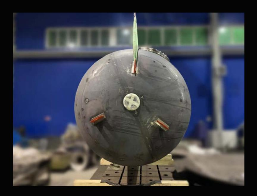
Production of a carbon sorption filter with the stainless steel frameworks, binding, shut-off valves and electric drive for Gazprom Energo, LLC.
